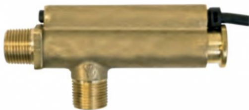
Fluxostat horizontal-vertical, 250bar, 30l/min, 75°C, 230V, 3A, IP 55, câble 1250mm
